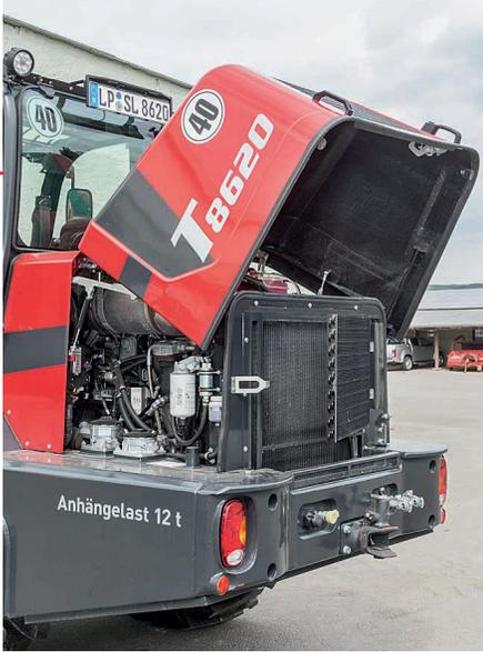
The 3.6-litre, four-cylinder Deutz motor is Stage IV compliant. It is available with three power outputs of 75kW/102hp to 100kW/136hp.
