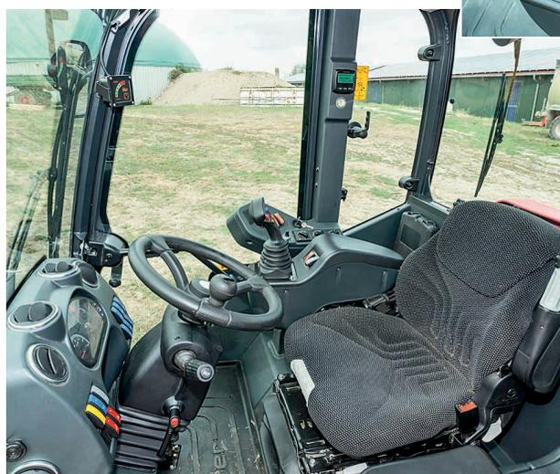
The ignition key and ventilation control have moved to the right. Next to them is the optional dial that sets the engine speed when in drive pedal mode.
