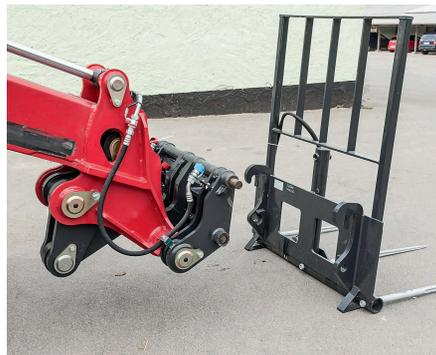
The boom has a sturdy Z-bar linkage that develops 4.2t lift force and 5.2m lift height. An interesting feature, although not common in the UK/Ireland, are the double hooks on the attachments which offer two different angles.
