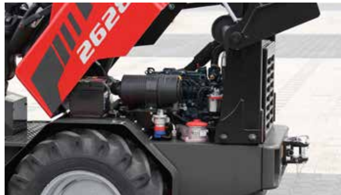
The motor room opens forwards. This makes all service points easily accessible from both sides of the machine.
