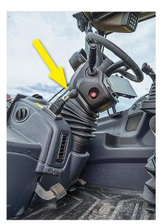
The handbrake control has been relocated to the left of the loader's steering column, which is adjusted using a foot pedal.
