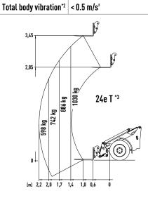
$^{\ast 1}$  boom horizontal, not extended, with pallet fork (acc. to ISO 14397)  $^{\ast 2}$  according to ISO 8041
