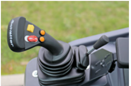
Joystick with expanded functionality
