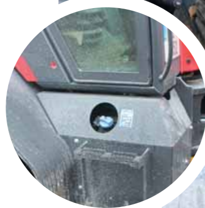
Above inset: The machine's AdBlue tank is conveniently located behind the offside cabin access steps, which makes for convenient refilling
