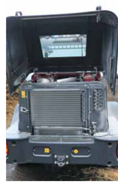
Left: Rear cooling radiators have the option of being specified with a reverse fan function
