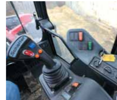
Above: The main control console incorporates a new joystick design that controls all main loader and attachment functions as well as direction of travel
