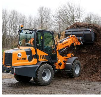
Unlike a classical wheel loader, the telescopic wheel loader has a much larger reach, piling up woodchips into high heaps, for example, to save storage space.
