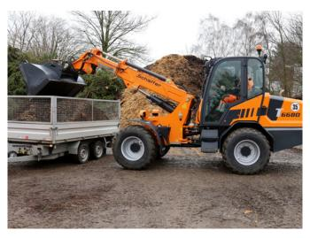
One of the typical tasks of the telescopic wheel loader – telescoping to a 4.95m height at attachment pivot pin, even larger trailers and trucks can be filled without difficulty..
