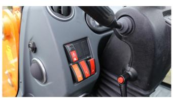
At a flick of the switch, the telescopic wheel loader is set to platform operating mode and this triggers a number of safety functions.
