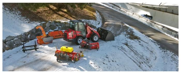
The large selection of attachments allows for versatile use: Snow blade, roller spreader and snow blower are primarily needed in winter. The pallet fork, the large-volume universal bucket and the sweeping machine assist in logistical tasks and maintenance work around the bobsleigh track.
