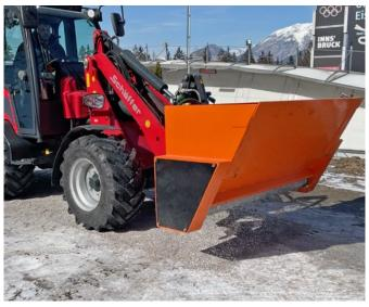
The roller spreader enables a homogeneous spreading pattern with a fixed spreading width in combination with the loader's cruise control.
